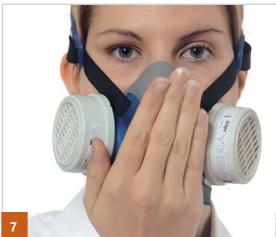
Positive pressure test: Seal the exhalation valve of half mask and exhale. The half mask will inflate slightly. If the exhaled air leaks out of the mask, readjust the face piece and adjust the straps or use a different mask size. Repeat test until a successful seal check is met.
