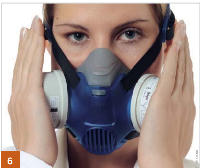
Negative pressure test: Seal both respiratory filters with your hands and breathe in until a negative pressure (suction) is generated. Hold your breath for a moment. The negative pressure should be maintained. If not readjust the face piece and adjust the straps or use a different size of mask. Repeat test until a successful seal check is met.
